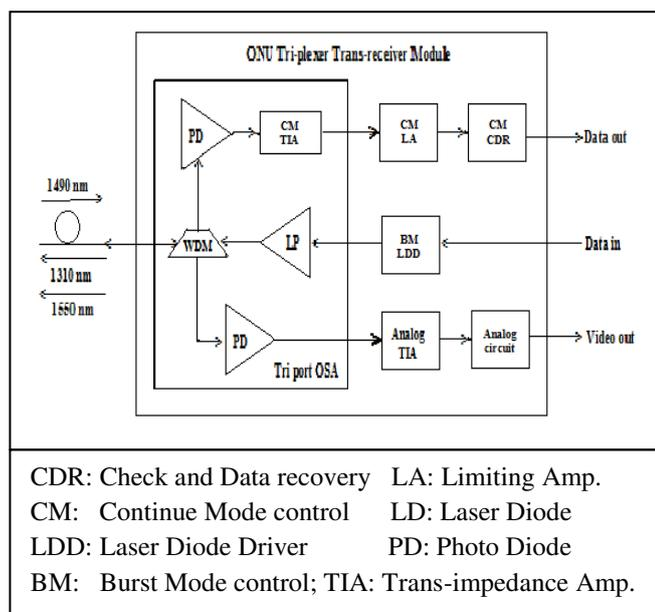
Figure 2. Functional block of the GPON ONU tri-plexer Trans- receiver module setup.
