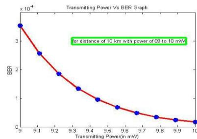
Figure 4(a): For 10 km distance with 09 to 10 mw transmitting power.
