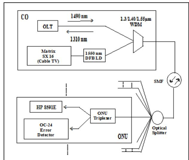
Figure 1. The GPON Trans- receiver module setup for measurement
